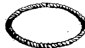
Twisted O-Ring: Installed Wrong
