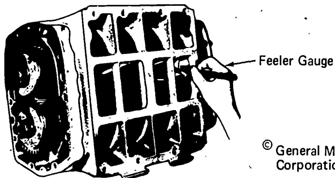
Measuring End Clearance Between Blower Rotors and End Plate
