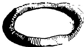
Swollen O-Ring: Use of Wrong Fluid
